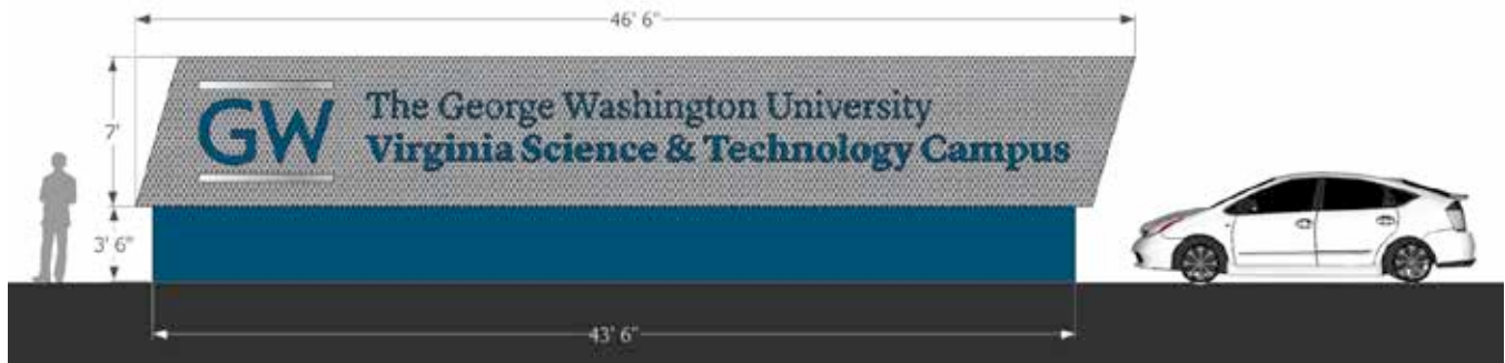
Illustrative Graphic Depicting Approximate Maximum Sign Size for Type C Campus Monument
