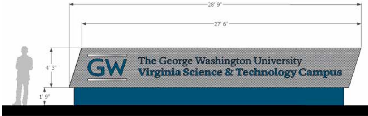
Illustrative Graphic Depicting Approximate Maximum Sign Size for Type B1 Campus Monument
