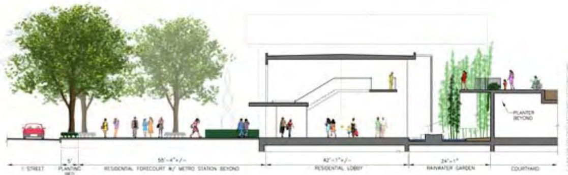
SECTION D-D @ RAINWATER GARDEN & RESIDENTIAL LOBBY SCALE: 1/8"=1'-0"
