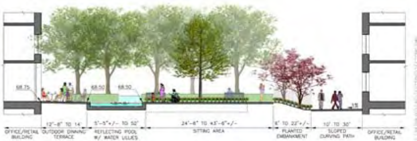
SECTION C-C @ COURTYARD SCALE: 1/8"=1'-0"
